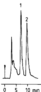
Fig 4 Separation of the enantiomers of MND Column \alpha_1 -AGP (100 mm \times 4.0 mm I.D.) Mobile phase phosphate buffer of pH 7.0 (0.01 M phosphate) containing 0.1 M sodium chloride and 7% (v/v) 2-propanol Flow-rate 0.3 ml/min Peaks 1 = ( R )-MND, 2 = ( S )-MND (0.008 a.u.f.s.)
